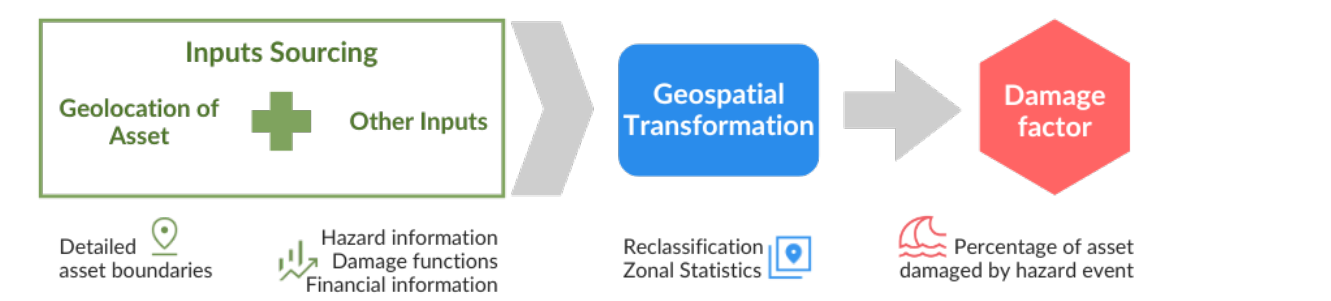
Figure 1: General approach for calculating physical hazard risks
